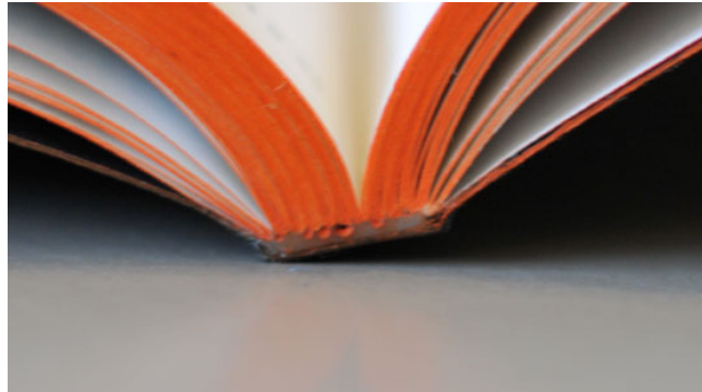
Figure 10: Perfect Binding with Sewed Hotmelt
